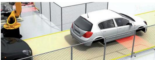
Access protection without muting initially saves muting sensors and hinged doors. The easy assembly enhances process safety.
