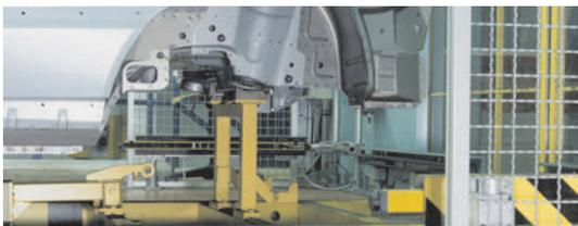
Object pattern recognition for individual settings of a defined object like complex skid constructions of a car.
