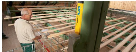
Reduced resolution: With C4000 Fusion machinery does not stop before the upper part of the body is detected.
