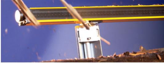
Falling chips do not trip the safety light curtain.
